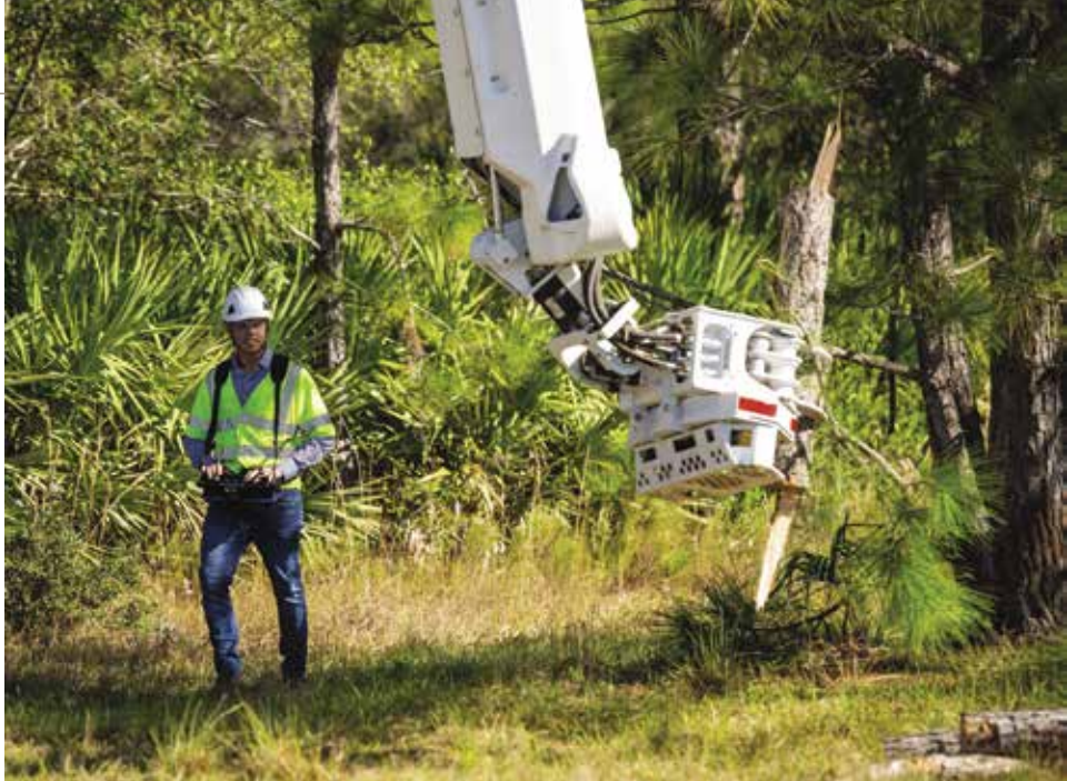
▲ FPL recently introduced a robotic trimmer to assist in tree trimming and vegetation management activities.
