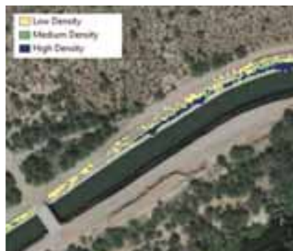
Figure 4. Vegetation density on the north side of an embankment slope
