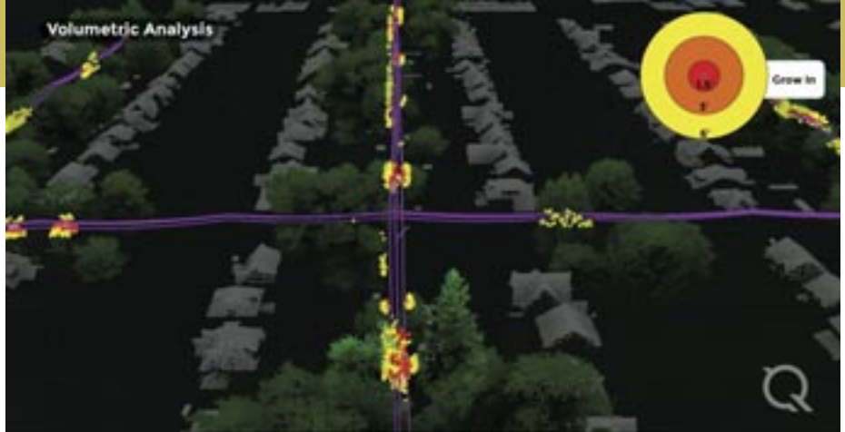
Figure 6. Red, orange, and yellow LiDAR returns designate the cubic feet of vegetation required to be removed on a multiple spans of distribution wires. This cubic assessment assists work planning, contract negotiations, and contractor auditing.
