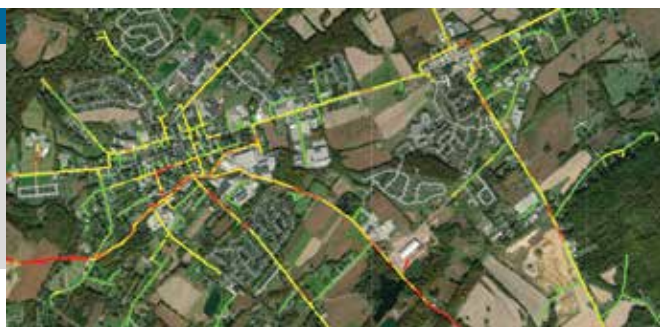
Image from the FirstEnergy TOP model, which was created using outage history; inspection records; weather history; and data related to soil, slope, etc. to inform VM decisions.
