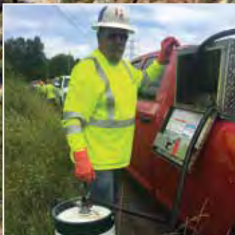
Hamilton Land Services has converted all application vehicles to a direct-connect, closed-loop system. Photo courtesy of Jerad Hamilton, Hamilton Land Services.
